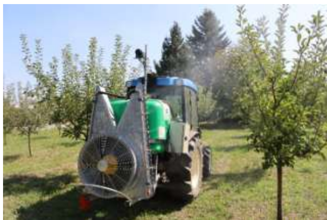
Fig. 5. Spraying equipment provided with automatic system for detecting the characteristics of the target culture
